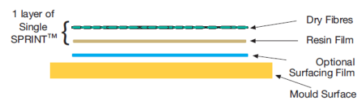
Cross-section of 1 ply of Structural SPRINT™
